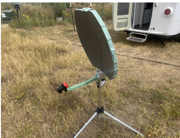
receive dish antenna with LNB
