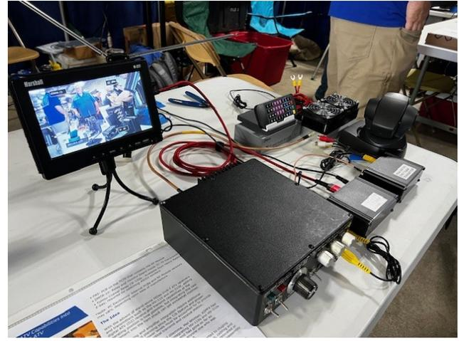
The 23cm transmitter cross-linking to the W8BI repeater was accomplished through use of an HV310 transmitter, a Jim Andrews, KH6HTV, 23-11A amplifier that was being used as a driver to drive an XRF-286, W6PQL amplifier
