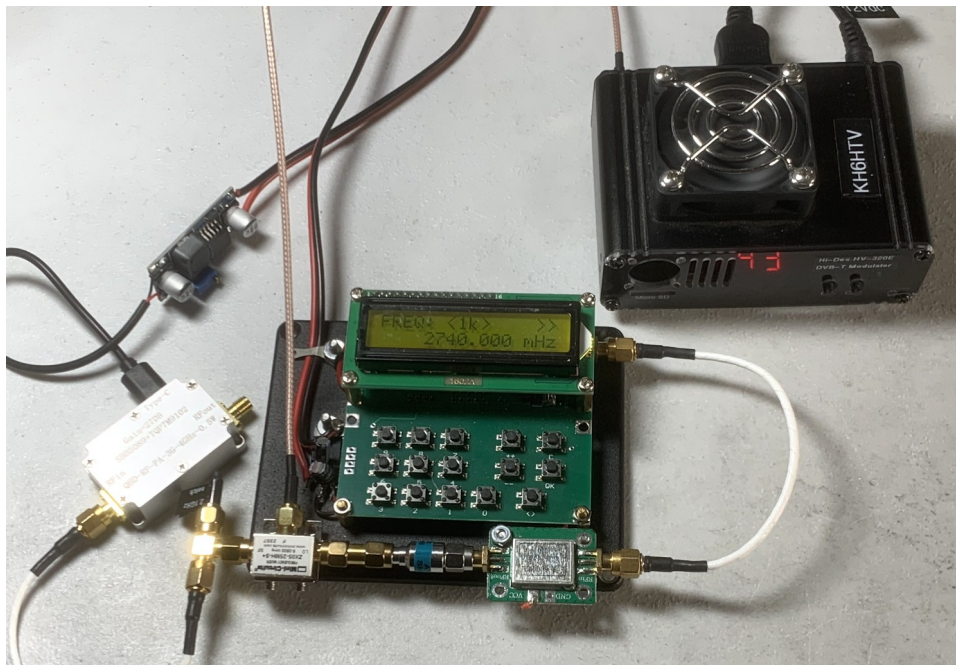
9 cm, DVB-T, 40 mW, Transmitter
