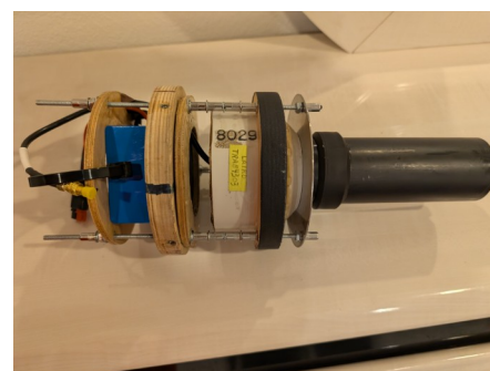
The electronics package complete with video camera, ATV transmitter, battery and antenna
