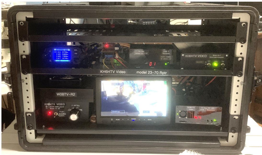
Fig. 1 This photo shows a proto-type 23cm to 70cm cross-band repeater. All the components were assembled onto two 1U, 19", relay rack shelves. This proto-type used the 70-9B, 10 Watt, rf power amplifier. It also included a 2m FM receiver, ABOMY - Arduino DTMF decoder / relay, video monitor and +13.8Vdc power supply.
