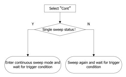
Figure 2-9 Process of Continuous Sweep
