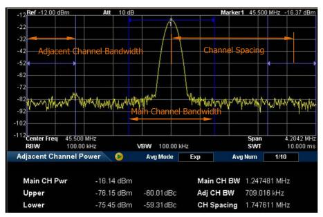
Figure 2-15 Adjacent Channel Power Measurement Interface
