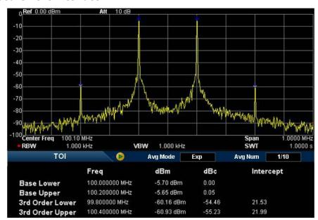
Figure 2-21 TOI Measurement Interface
