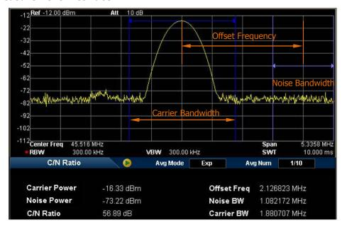
Figure 2-19 C/N Ratio Measurement Interface
