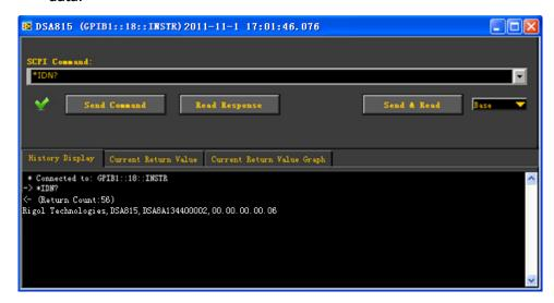
Figure 3-10 Write and Read Commands via GPIB
