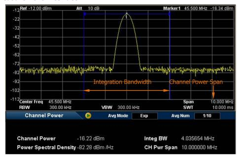
Figure 2-16 Channel Power Measurement Interface
