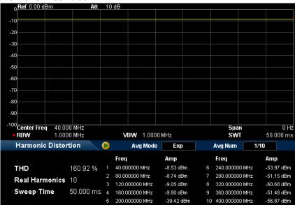
Figure 2-20 Harmonic Distortion Measurement Interface
