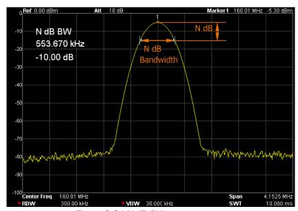
Figure 2-24 N dB BW measurement
