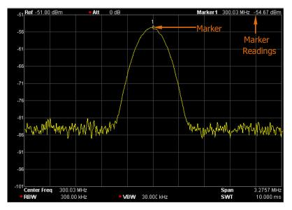
Figure 2-22 Schematic of the marker
