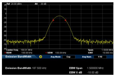
Figure 2-18 EBW Measurement Interface
