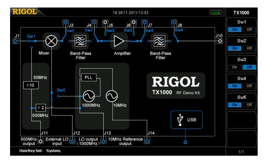
Figure 2-30 TX1000 control panel
