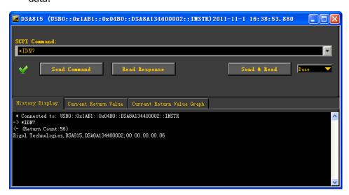
Figure 3-3 Write and Read Commands via USB
