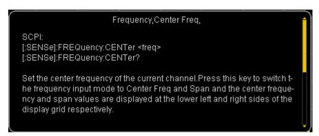
Figure 1-14 The Built-in Help Interface
