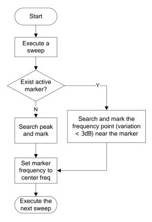
Figure 2-1 Process of Signal Track
