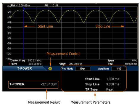
Figure 2-14 T-Power Measurement Interface
