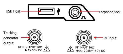
Figure 1-7 Front Panel Connectors
