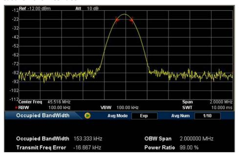
Figure 2-17 OBW Measurement Interface
