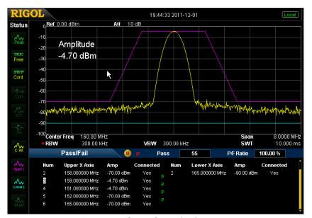
Figure 2-11 Interface of Pass/Fail Measurement
